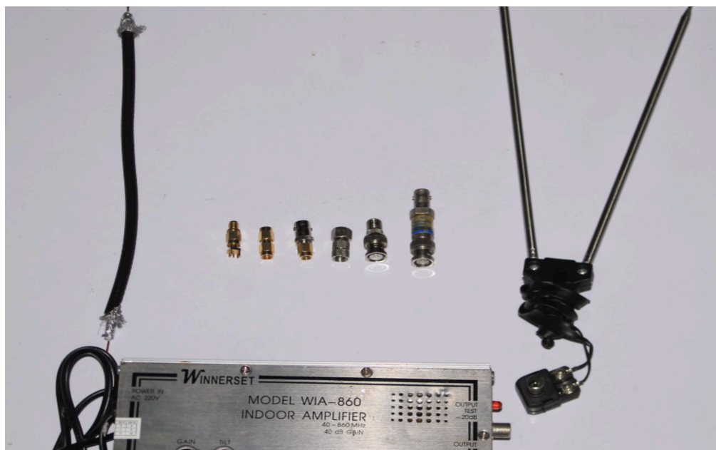
Figure 3.4: Cable Signal Amplifier, Connectors and Rabbit Ear Antenna.
